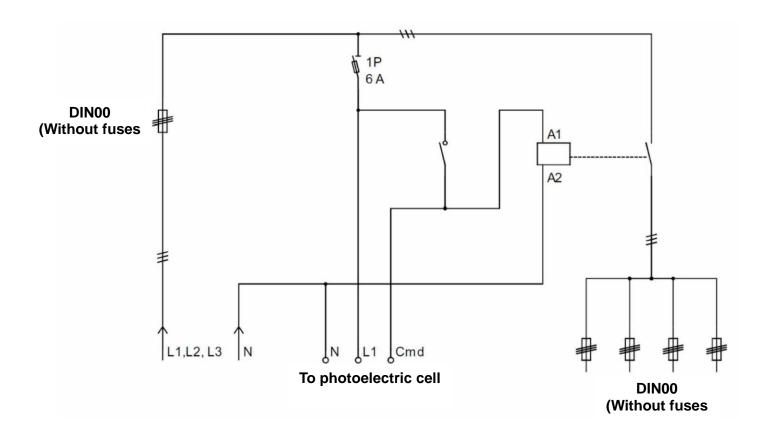
The power to the cabinet is normally provided from the Substation LB General Board or through distribution cabinets outputs, the outputs of this cabinet will be connected directly to public lighting poles.
